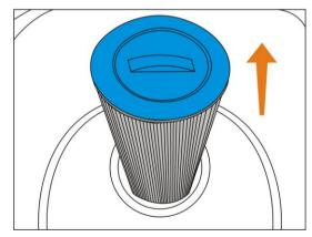
3. Place a new filter cartridge into the filter cylinder.
