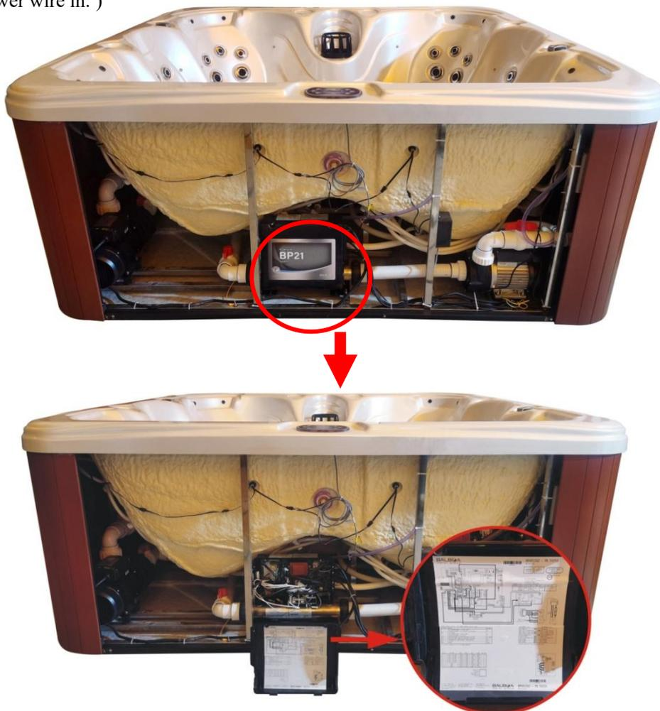
**Step 3:** If the drawings on the back of the control box cover mentioned in step 2 is not clear enough, please check the control box model above the control box, and then connect power wire according to the guides below
