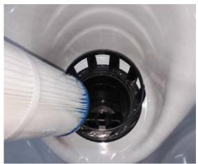
4. Place a new filter cartridge into the filter cylinder.
