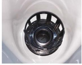
2. Hold the little handle and twist the filter basket part, and take out the part.
