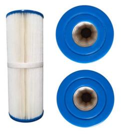
The filter cartridge needs to be checked, cleaned and replaced regularly. It is very important to keep proper water flow. A clean filter enables the hydrotherapy system to work properly and allows for more efficient filter cycles. Depending on the usage frequency of the spa, we recommend cleaning the spa filter cartridge every four weeks. If this is not done, the filter may block and restrict water flow, which causes improper filtration, poor jet performance and may possibly freeze.
